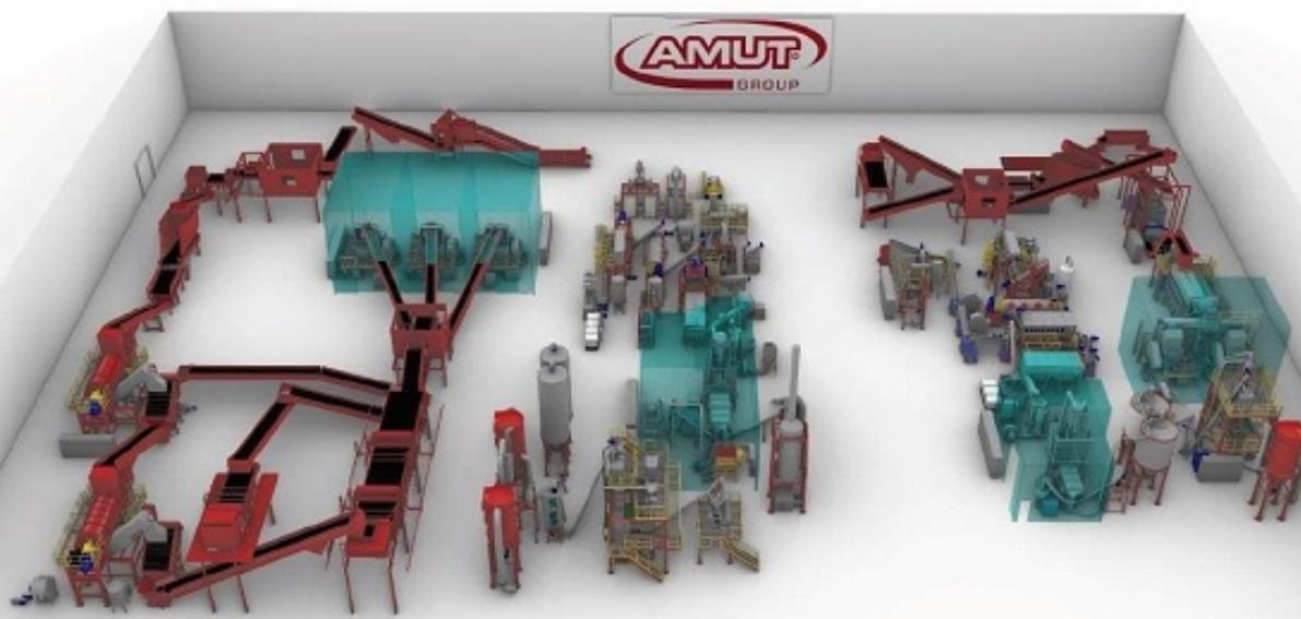
The lines, which will be processing light weight bottles with high percentages of PVC and non PVC shrinkable sleeves, will feature a double De-Labeller configuration. In the first stage the Amut patented De-Labeller performs a dry cleaning action able to detach most of the shrink sleeves labels while the second unit is a wet De-Labeller working as cold pre-washing, allowing to remove contaminants, without damaging the bottles and avoiding to lose the bottles necks during the process.
