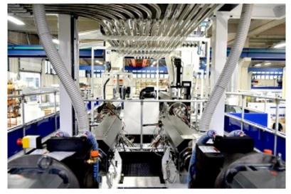
This new cast line has a very compact layout, available in a configuration starting from four extruders and five layers. The Polycast EVO lines boast primary level equipment thanks to the most prestigious suppliers and can be optionally equipped with our patented MDO IR1 (single stage) or MDO IR2 (double stage), which ensure the production of MOPP and MOPE film.
