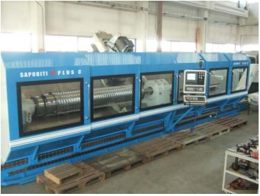
All the Electronic is Siemens and it is covered by 24 months worldwide warrantee. The CNC is the latest generation Siemens 840 DE. The machine important feature is that it can be equipped with an auxiliary milling head for disc cutter with a max. diameter of 200 mm. This head can be useful to work special screw profiles as cams, polygons, deep and narrow thread. This head has an auxiliary controlled axis for the inclination of the disc cutter.
