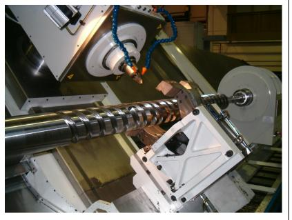
Maximum spindle speed: 6000 rpm, cutter motor power: kW 40. This motor for the milling head is sealed with internal water chilling circuit.
