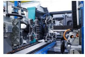
An X-Series Mini-Modula compact side-entry robot from Campetella used for the IML of plastic yoghurt cups made of polypropylene. The
