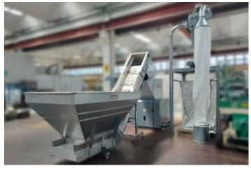
enclosed feed chute to granulator. The infeed conveyor is integral part of the system, not anymore an appendix or an auxiliary device, and is controlled by the granulator so to synchronize all operations in full.
